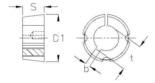
$\begin{array}{lll} b & = 10 \\ Bore & = 38 \\ Bush type & = 3030 \\ D1 & = 108 \\ S & = 76,2 \\ Screw size & = 5/8 \times 1 \ 1/2" \\ t & = 41.3 \end{array}$
